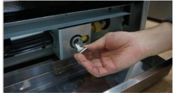
For 30-inch gas range and 36-inch gas range, connect the gas line (adaptor) to the gas inlet but not the cap for NG/LP Conversion;
