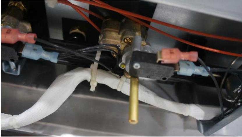
h. Using a flat screwdriver, replace gas valve bypass jets with bypass jets for LP;
