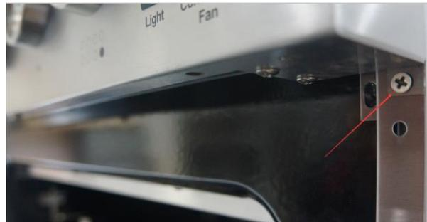
f. Screw out the 5 screws from the top of the control panel support;
