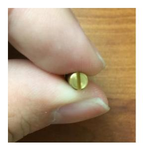
NG bypass orifice has a number on the side; LP bypass has nothing on the side.
