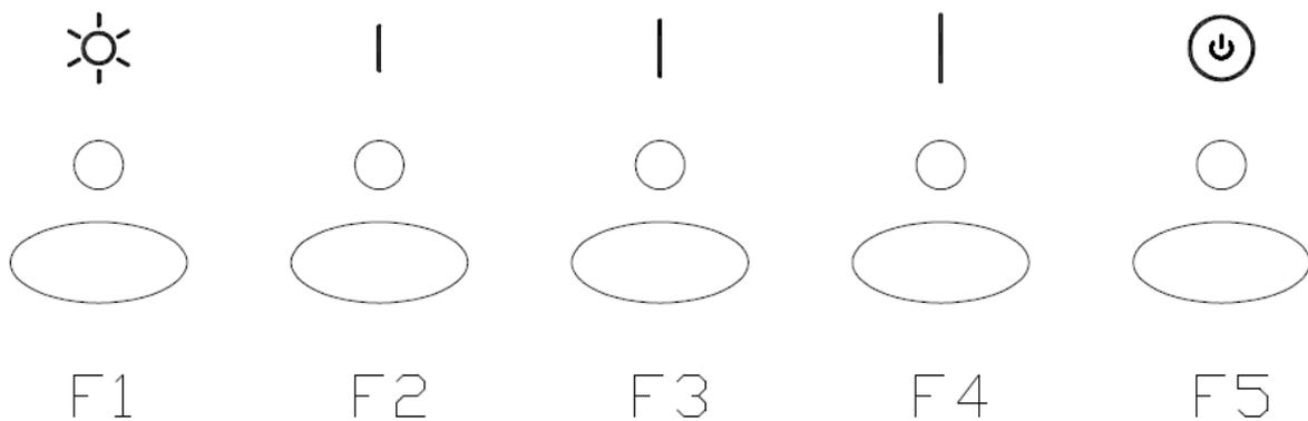
**Function Button:** LED light button F1 low speed F2 medium speed F3 high speed F4 time-delay/on-off F5
