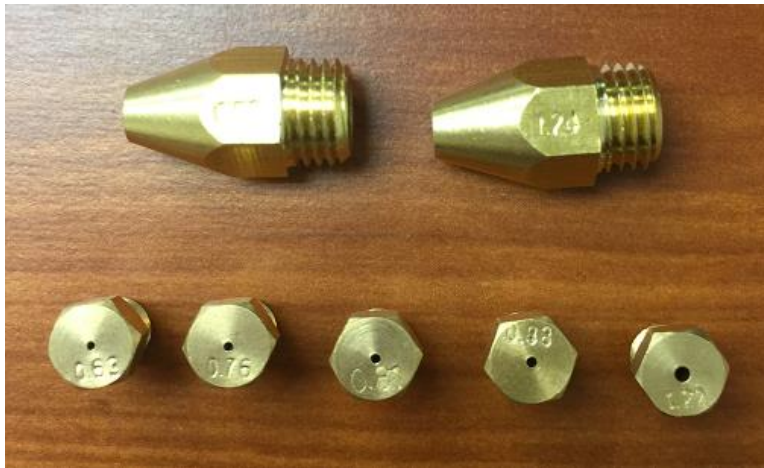
Top: Orifice for Oven Broiler Burner / Oven Burner Bottom: 4000BTU/6000BTU/8000BTU/9000BTU/18000BTU Top Burner Orifice
